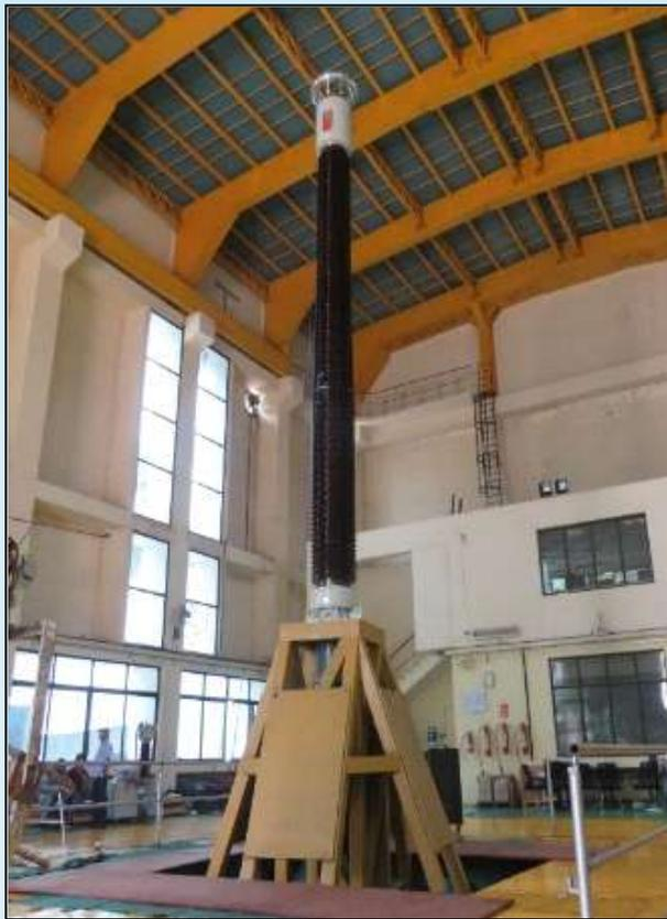
The Earthquake Vibration Research Centre, CPRI successfully carried out seismic qualification test on 800kV, 2500A condenser bushing with air and oil-end porcelain insulator mounted on support structure. The test was performed for M/s. CG Power and Industrial Solutions Limited, Nasik.
