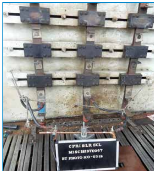
Short-time current test at 5.0kA rms for 10 seconds (symmetrical) was carried out on 17.2 mm dia 700 mm Long Copper Bonded MS Rod
