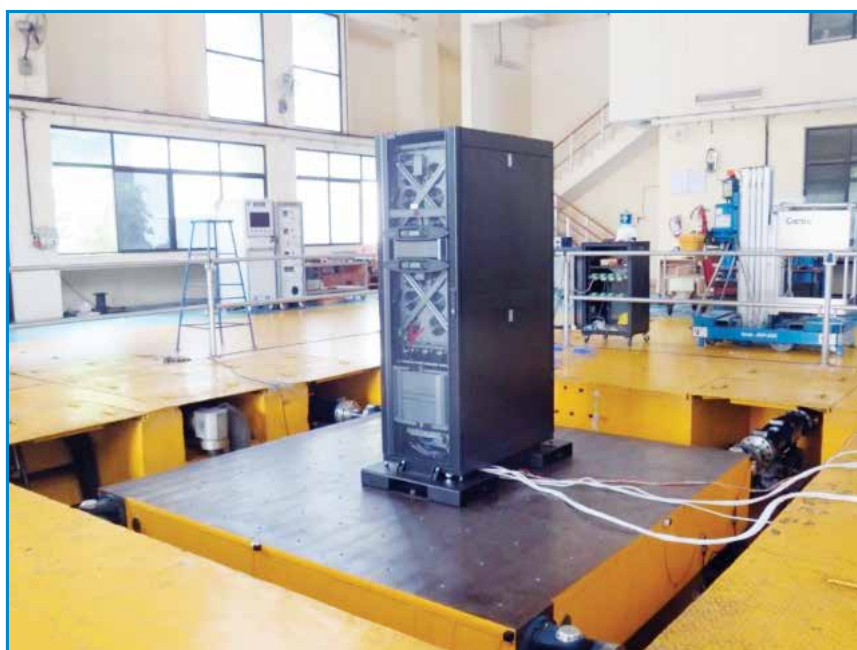
Seismic qualification test on Smart Uninterrupted Power Supply 20 KVA
