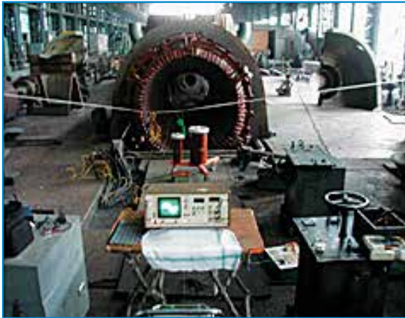
Partial Discharge test on 110 MW Turbo Generator
