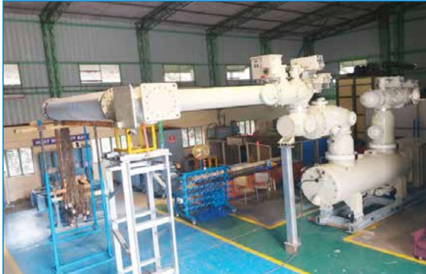
Temperature rise test on 245kV and 420kV GIS
