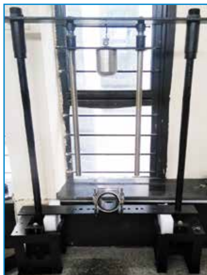
Stress testing on 400kV, 2500sq.mm cable cleats for M/s. PTE (Power Transmission and Telecommunication Equipment) Factory Co., Jeddah
