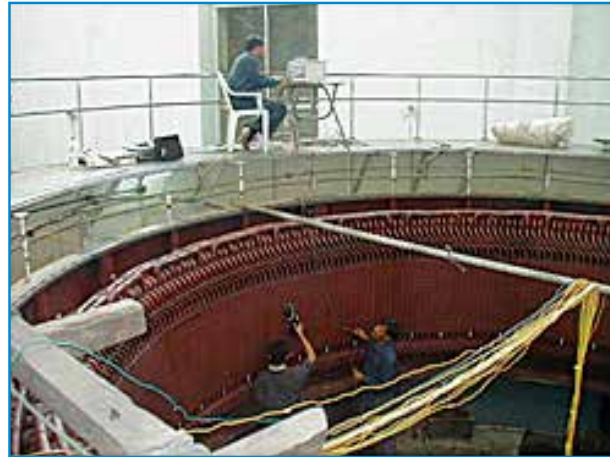
ELCID Test on Hydro Generator
