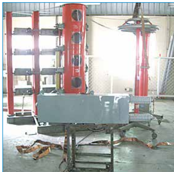
Test arrangement for Lightning Impulse voltage test 1000kvar, 22kV, 6.9 \mu F Fuseless HT Capacitor unit
