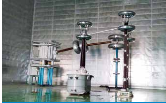
Partial Discharge test on 420 kV OIP condenser bushing
