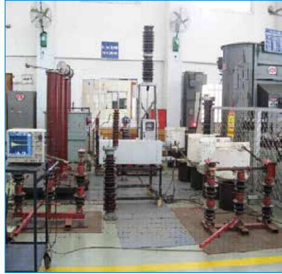
Arrangement for Discharge Current Test on 778.41kvar, 12.56kV, 50Hz, 1 Phase Fuseless Series capacitor
