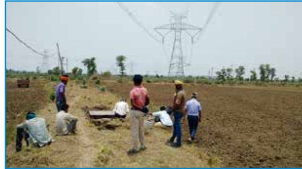
Measurement of Ionic current density from \pm 800 kV, HVDC Champa-Kurukshetra line of PGCIL
