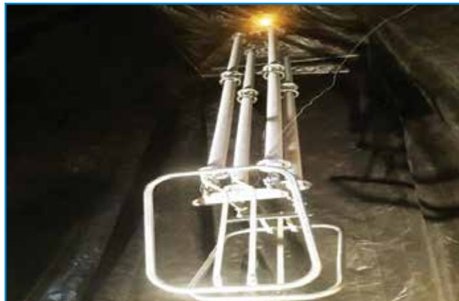
DC Pollution Test by Solid -Layer method on \pm 500 kV HVDC Composite Insulator String
