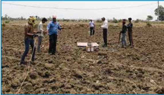
Measurement of Ionic current density from \pm 800 kV, HVDC Champa-Kurukshetra line of PGCIL
