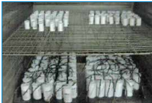
Some of the AC Motor capacitors tested
