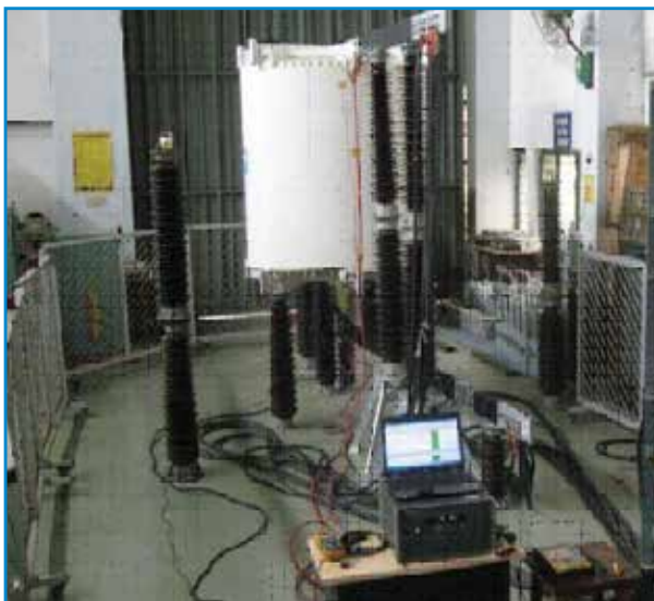
1.0mH, 2000A, Line trap undergoing temperature rise test
