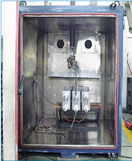
Arrangement for Thermal Stability Test on 778.41kvar, 12.56kV, 50Hz, 1 Phase Fuseless Series capacitor
