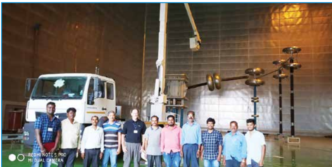
Dielectric test on truck mounted insulating boom
