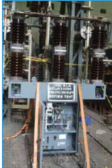
Electrical endurance test on 36 kV, 1600 A, 26.3 kA, Outdoor PCVCB
