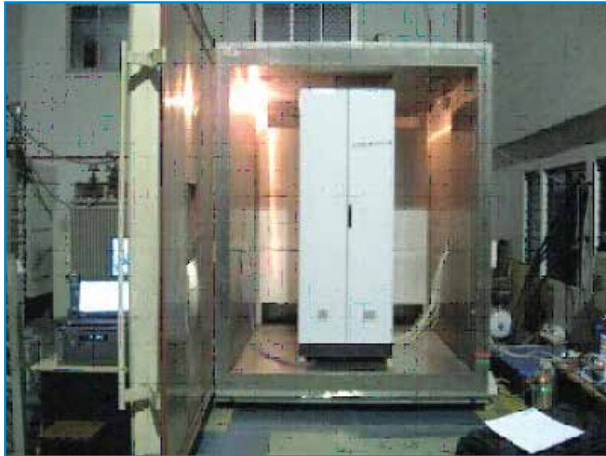
A view of the D-EHC panel undergoing tests
