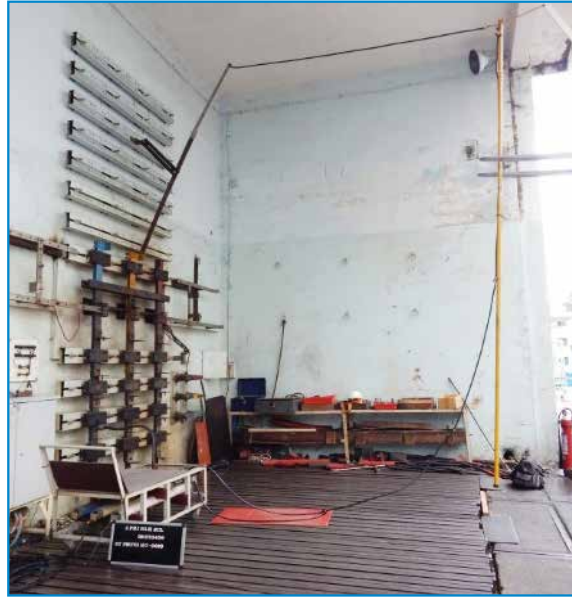
Short-circuit test at 6.25kA rms. for 1.0 second on Discharge Earthing Rod assembly
