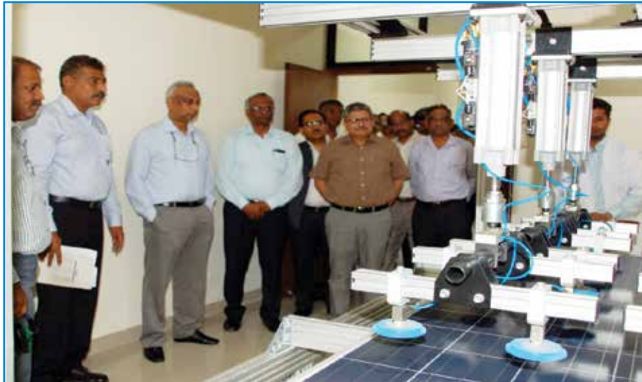
Demonstration of Mechanical Load Impact Test on SPV module
