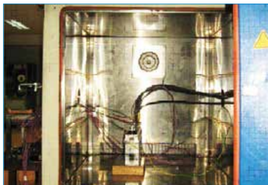
Power electronic capacitor from Spain tested for thermal stability test
