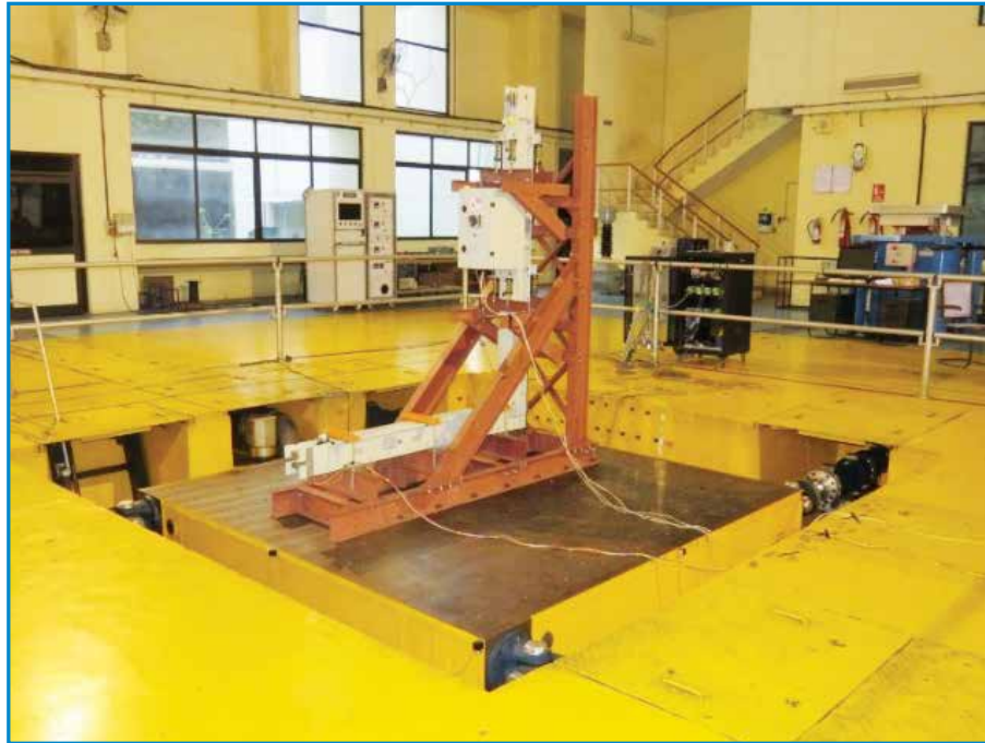
Seismic Qualification test on Sandwich busway system
