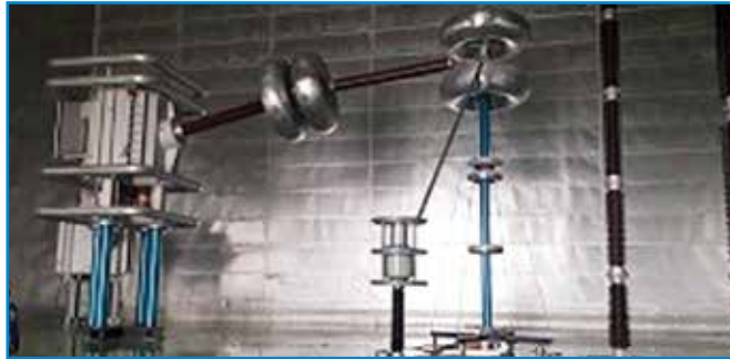
Partial Discharge test conducted on 145 kV. live tank Current Transformer
