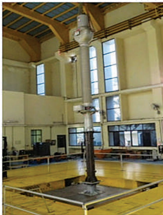
Seismic qualification test on Current Transformer
