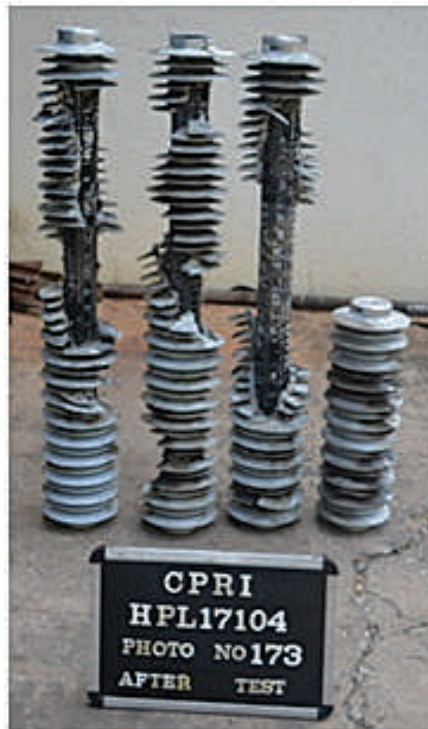
Short-Circuit test on Surge Arrester
