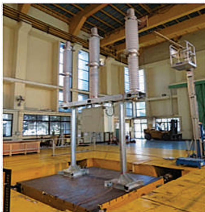
Seismic qualification test on three pole operated Circuit Breaker
