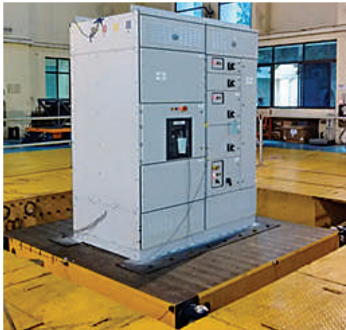
Seismic qualification tests on 440 V Low voltage switchgear
