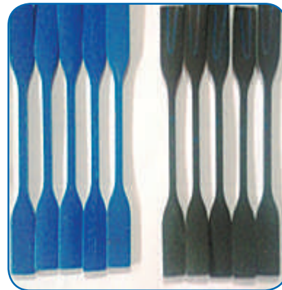
Change in color of cable outer sheath from before color of blue to after UV ageing color of black
