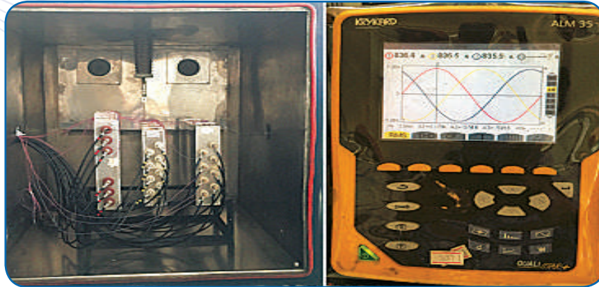
A view of the test set up for conducting thermal stability test on 9000 \mu F-2.8kV DC, 7500 \mu F-2.8kV DC and 7500 \mu F-2.8kV DC Power electronic capacitors simultaneously at 835 Amperes
