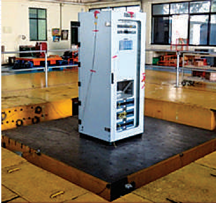
Seismic qualification tests on Integrated Motor Control System Panel
