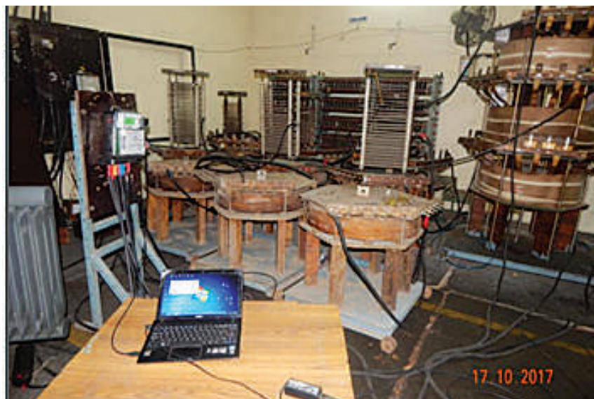
“Influence of Short time overcurrent test on Smart Meters- First Time Test at Short Circuit Laboratory, CPRI, Bangalore”
