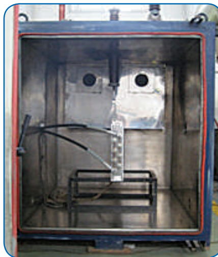
Power electronic capacitor of rating 7.5 mF which underwent destruction test in the Capacitors Division for the first time
