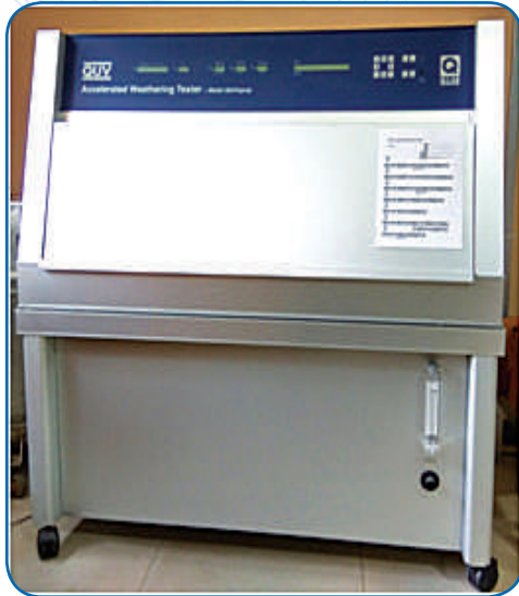
Photograph of the UV test chamber using Fluorescent lamp
