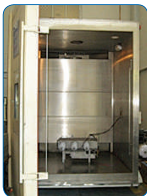
A view of the tested 3 \Phi , 27kV, 630A Load Break Switch in the Capacitors Division
