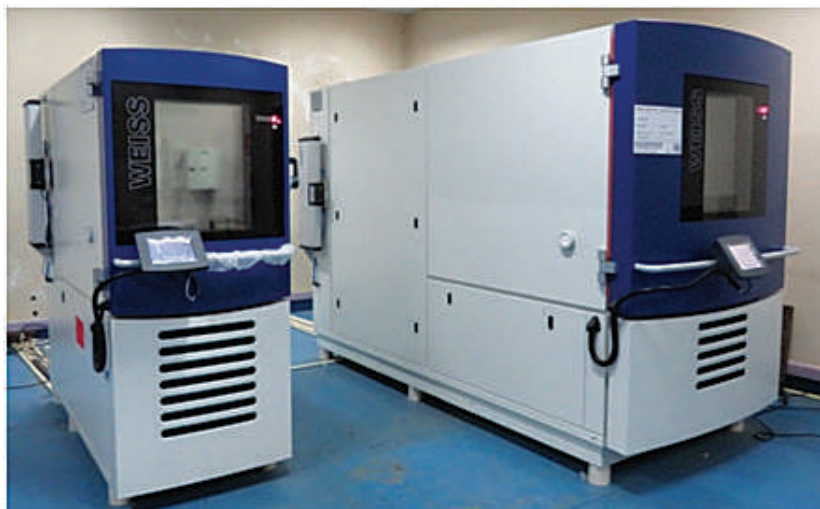
Temperature and Humidity Chamber, Volume – 250 Liters & 800 Liters
