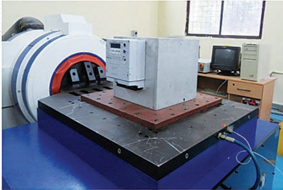
Vibration and shock testing of Smart Energy Meter
