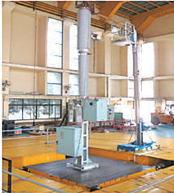
Seismic qualification test on Circuit Breaker
