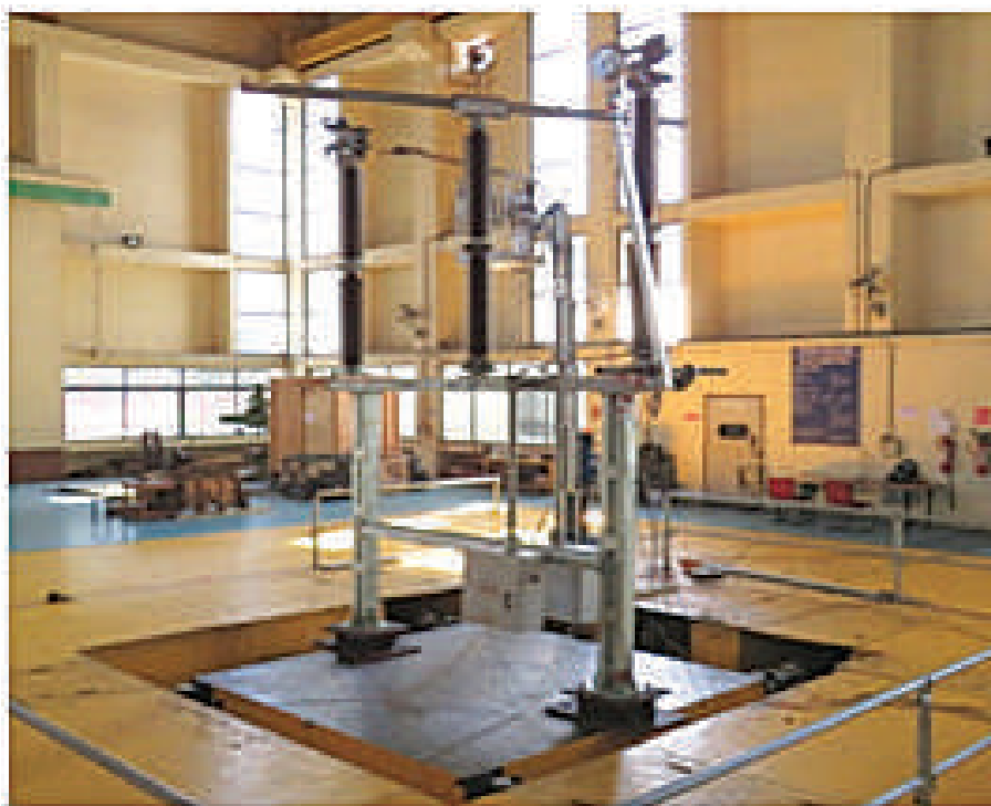
Seismic qualification test on Horizontal Double Break Disconnecter
