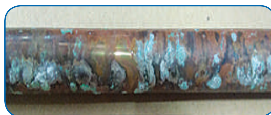
Portion of earth rod post corrosion test in sulphurous atmosphere
