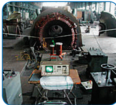
Partial Discharge test on 110 MW Turbo Generator
