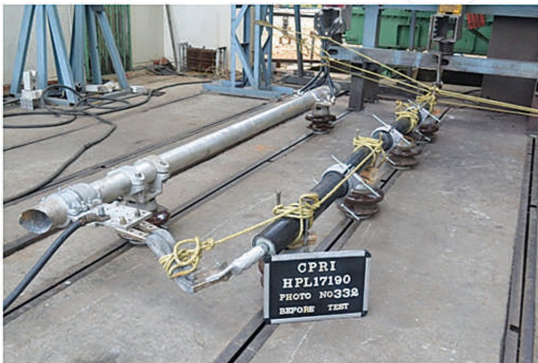
Short time current test on Cable Cleat
