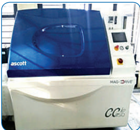
Cyclic corrosion test chamber at Insulation Division
