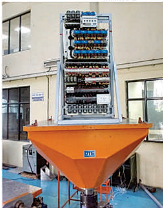
Vibration and shock testing of Relay Panel
