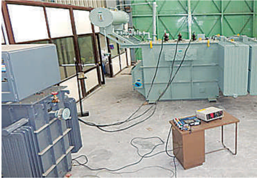
Temperature rise test on Distribution Transformer for the first time at Short Circuit Laboratory, CPRI, Bangalore
