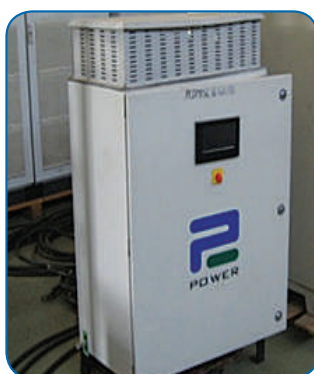
Active Harmonic Filter(AHF) undergoing tests in the Capacitors Division
