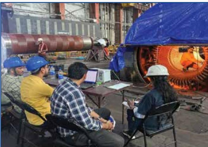
Winding Resistance test at 250 MVA Generator
