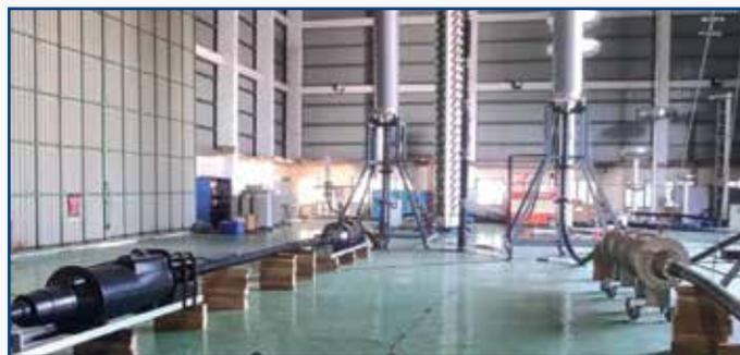
400 kV XLPE Cable system set up for Load Cycle Test
