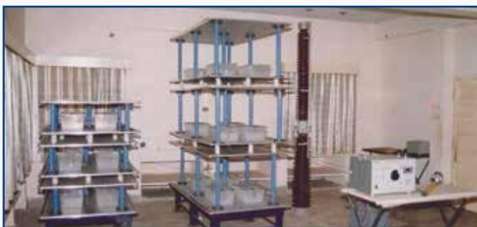
**Figure 2:** Electric field exposure test facility for mice, rats and seedlings
