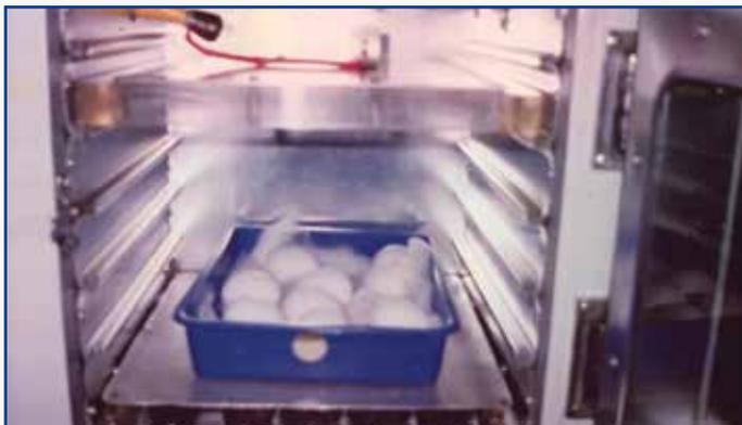
**Figure 3:** Electric field exposure test facility housed in an incubator for chick embryo
