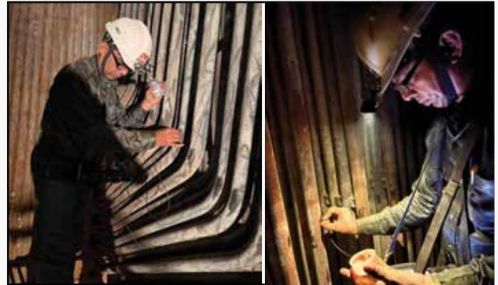
Thermal Research Centre (TRC), CPRI, Nagpur carried out the Magnetic Particle Inspection (MPI) & Ultrasonic Testing (UT) for compressor diaphragm, thrust bearing and journal bearing in Unit No.1 for M/s. NEEPCO, AGBPS, Bokuloni, Assam.
