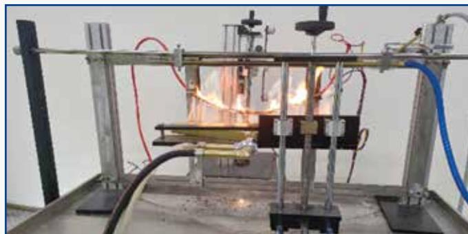
Test for Resistance to Fire with mechanical shock for fire survival Cable
