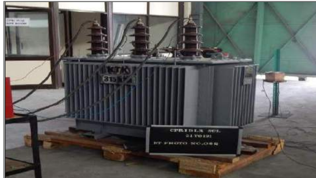
Temperature-rise and Determination of sound level tests on 315kVA 33000/400V Three Phase Distribution Transformer
