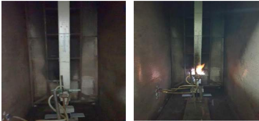
Resistance to Flame Propagation test on Sandwich Busway
