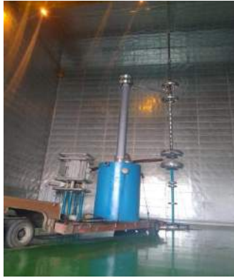
800kV RIP Transformer Bushing undergoing Partial Discharge test
