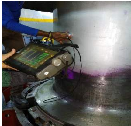
Ultrasonic testing of turbine shaft in progress
