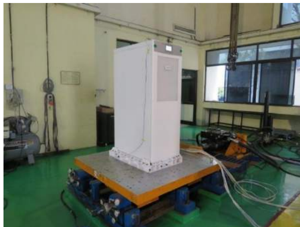
Vibration testing of Electrical Panel
