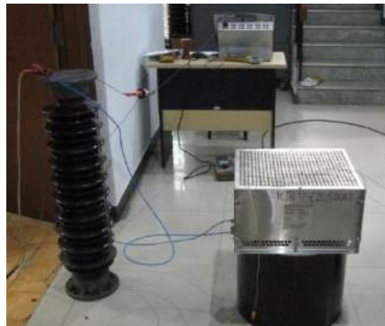
A view of the test arrangement for testing of Earth Discharge Resistor
