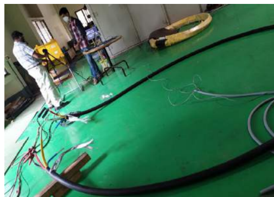
Remote/Virtual witnessing of type testing on 4 Core X 185 Sq.mm, Aluminum Conductor, XLPE insulated, PVC Sheathed 0.6/1 kV Cable
