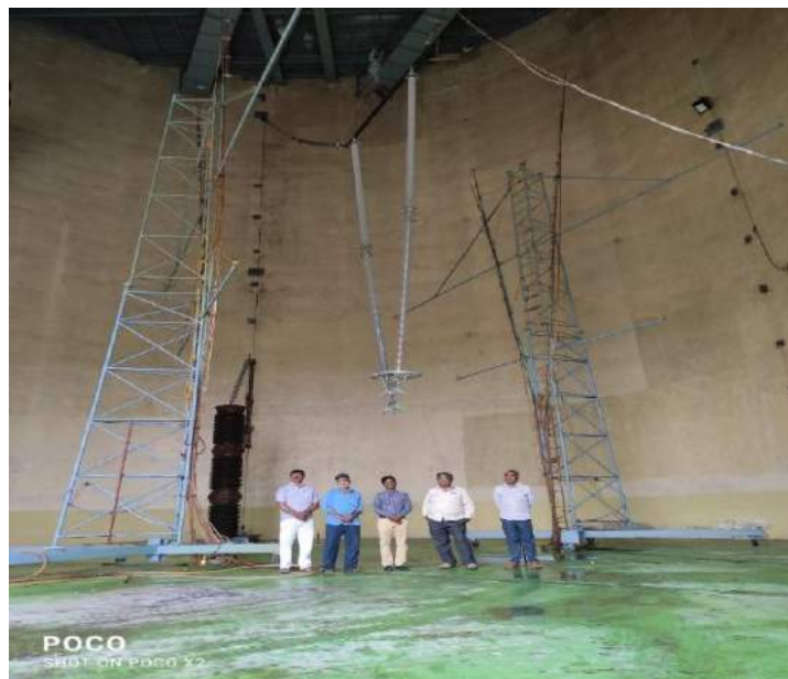
Artificial Pollution test using salt fog on 800 kV composite insulator of 9.2 Meter
