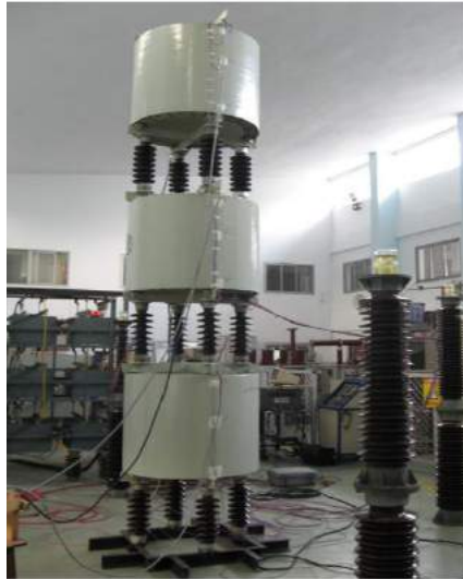
A view of the test arrangement for testing of Three Phase Reactor
