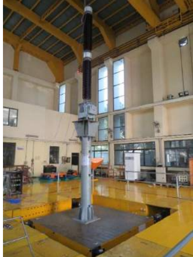
Seismic qualification test on 420kV Capacitor Voltage Transformer
