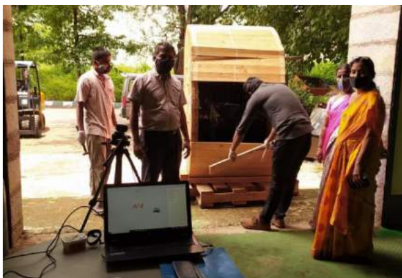
Remote/Virtual witnessing of type testing on 4 Core X 185 Sq.mm, Aluminum Conductor, XLPE insulated, PVC Sheathed 0.6/1 kV Cable
