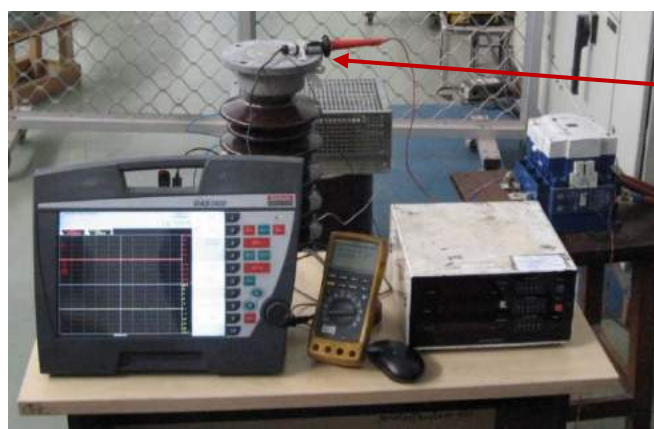
A view of the test arrangement for testing of Pre-charge Resistor
