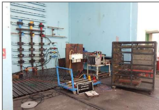
Making & Breaking Capacities test carried out at 4000A 1000V DC on 1000V 2000A 4 Pole DC Switch
