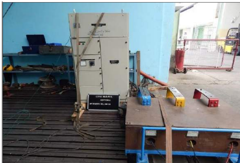
Verification of short-circuit withstand strength test at 35kA DC for 1 second on 250V 630A DC Distribution Board
