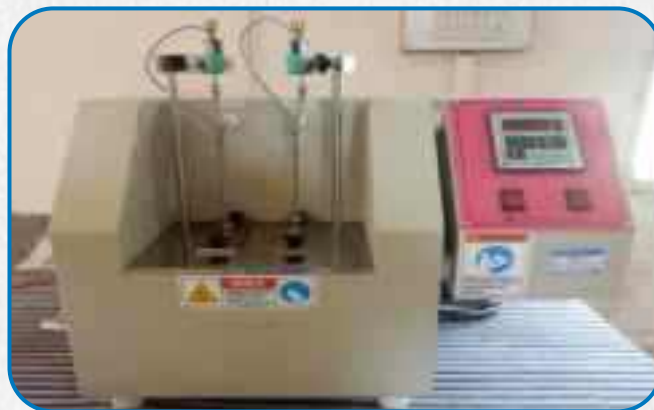
Head Deflection Test (HDT) on Material Strip of Meter Terminal Block
