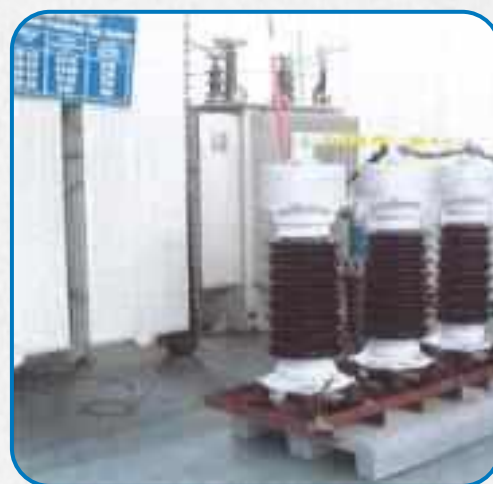
Over Voltage test on 0.217 F, 14.63kV - 3 Nos. Capacitor Divider Modules
