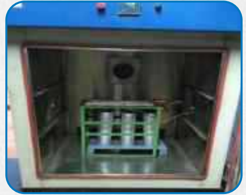
Thermal Stability test on 50kVAR, LV Shunt Capacitor
