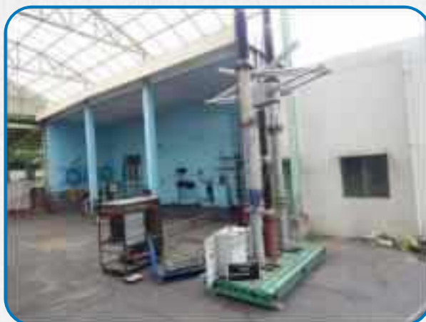
Bus-transfer current switching test on 245kV, 2000A Pantograph Disconnectors
