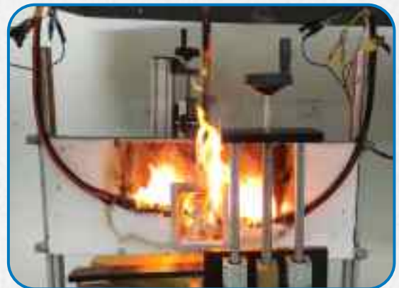
A view of GI LILO Box with Cable and connectors during test
