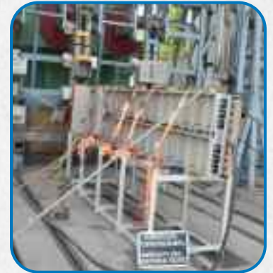
Short time withstand Current test on 1kV, 5000A, 100kA Busduct
