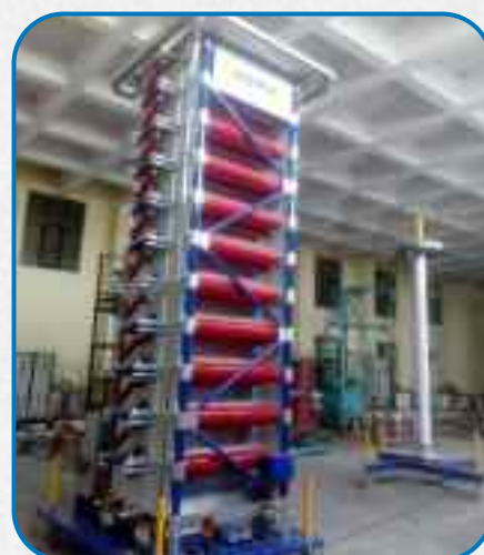
1000kV, 100kJ Impulse Voltage Generator
