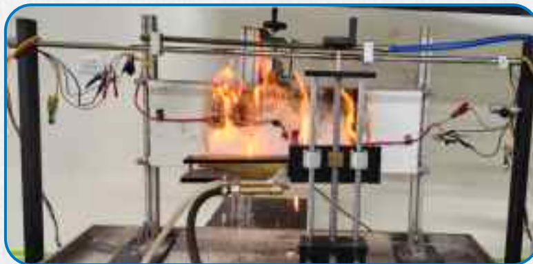
Resistance to Fire with Mechanical Shock on 2 Core X 1.5 Sq.mm, LSZH Sheathed 300/500 V Cable
