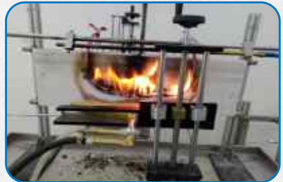
A view of Cable Sample during Resistance to Fire and Mechanical Shock test as per BS EN 50200
