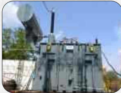
Short Circuit Testing of 500MVA, 1ph Station Transformer Unique Testing
