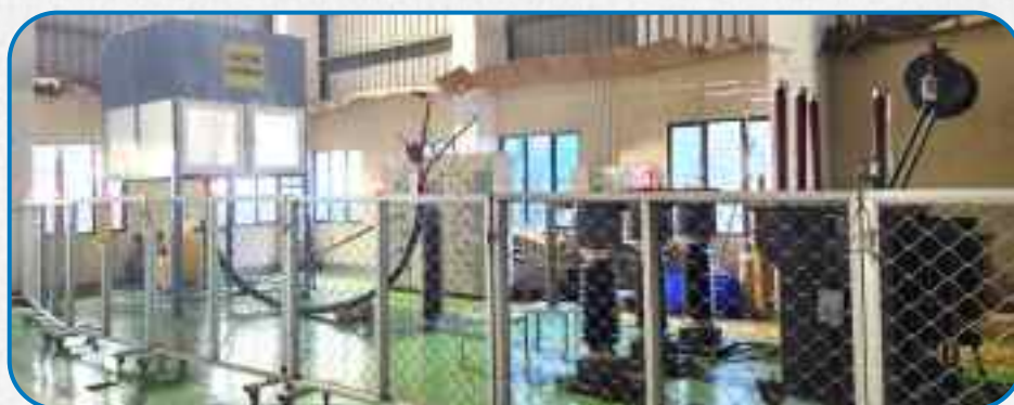
Salt Fog test on MV Cable Accessories as per IEC 60502-4
