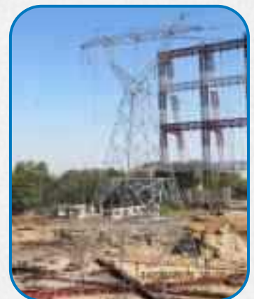
220kV Tower under Test
