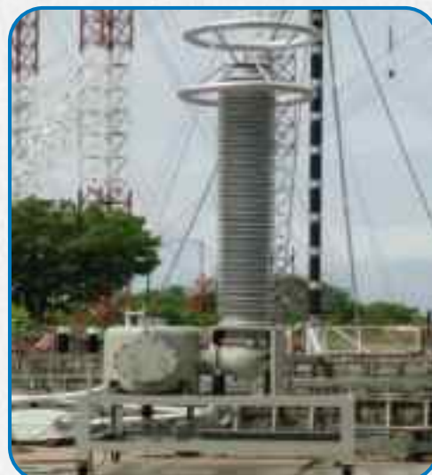
SF 6 puncture withstand test facility on Insulator
