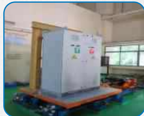
Vibration test on Top Panel of Wind Turbine
