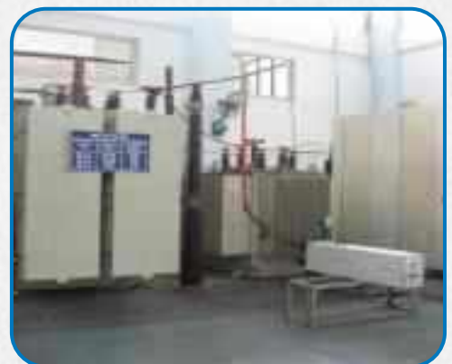
Over Voltage Test on 500kVAR, 8kV, Int. Fuse Capacitor Unit
