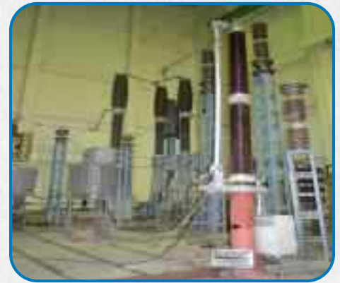
Induced Current Switching tests on Disconnector
