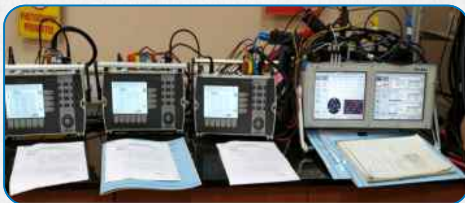
Calibration of three Portable Reference Standard Energy Meters
