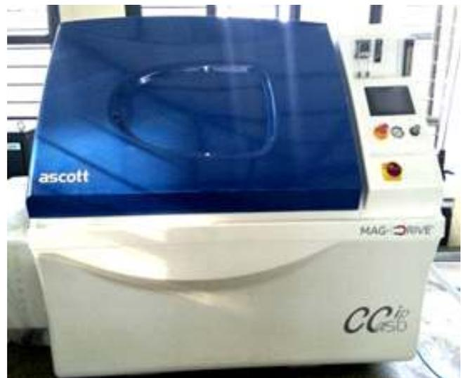
**Cyclic Corrosion Test Equipment**
