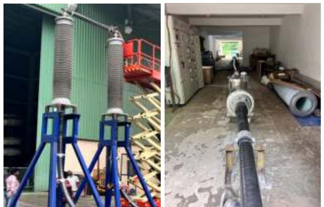
**Pre-qualification test arrangement - Fixing of terminations & laying of Cables with GIS Accessories for 220 kV Cable System**
