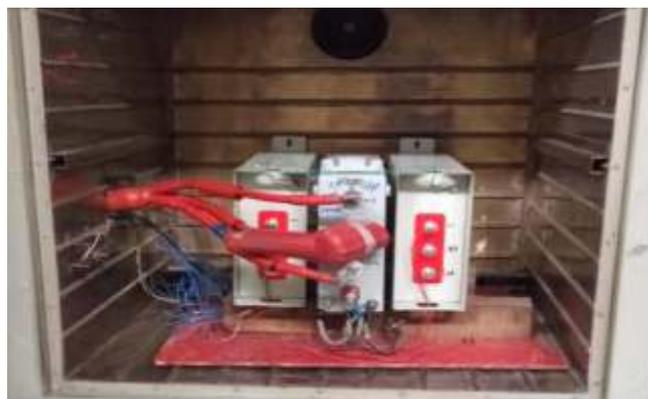
**Arrangement for Thermal Stability Test on 4.434kV 630kVAR, 3 x 85 MFD Capacitor**
