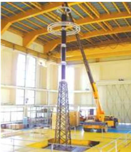
The Division is equipped with a Triaxial shake table of 3m x 3m size and 10 ton pay load capacity for simulating earthquake vibrations. In addition, the Division has Electrodynamics Shaker Systems for carrying out vibration tests on products and assemblies.
