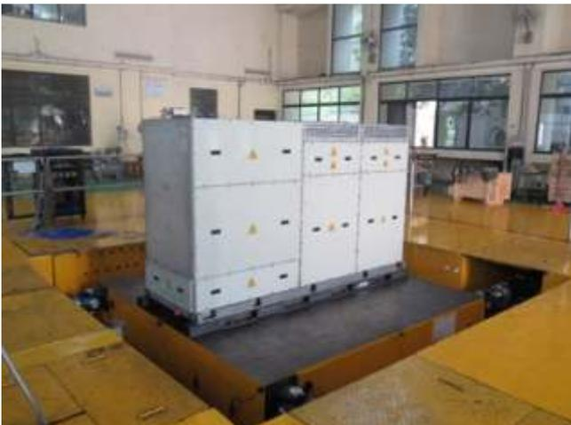
**Vibration test and Shock test on Traction Converter**
