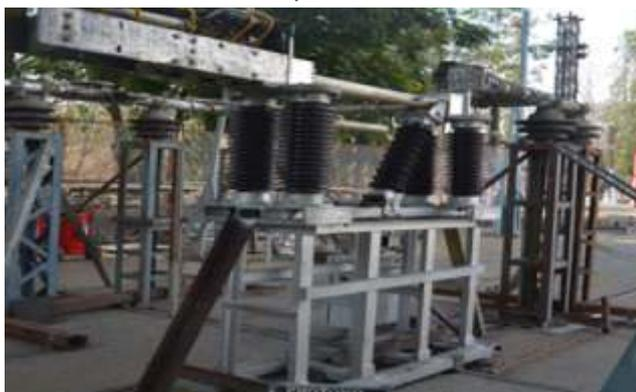
**72.5kV, Co-axial type disconnecter tested at 130kArms for one second with a peak of 325kA**
