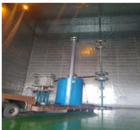
**800kV RIP Transformer Bushing under Partial Discharge test**
