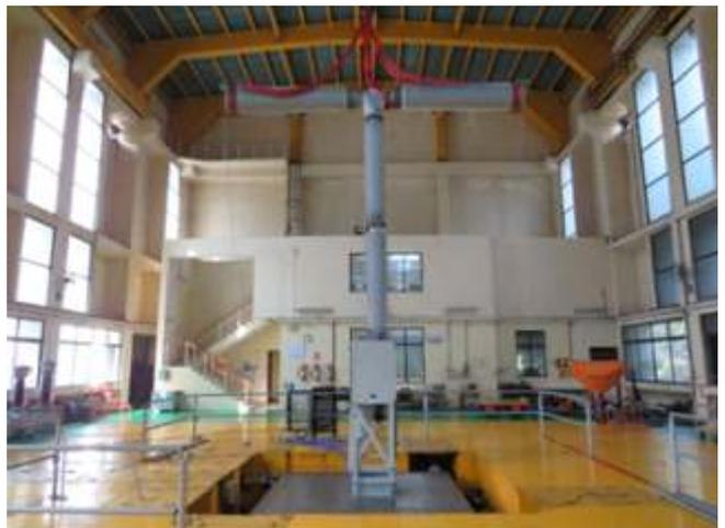
**Seismic Test on 420 kV Single Pole
