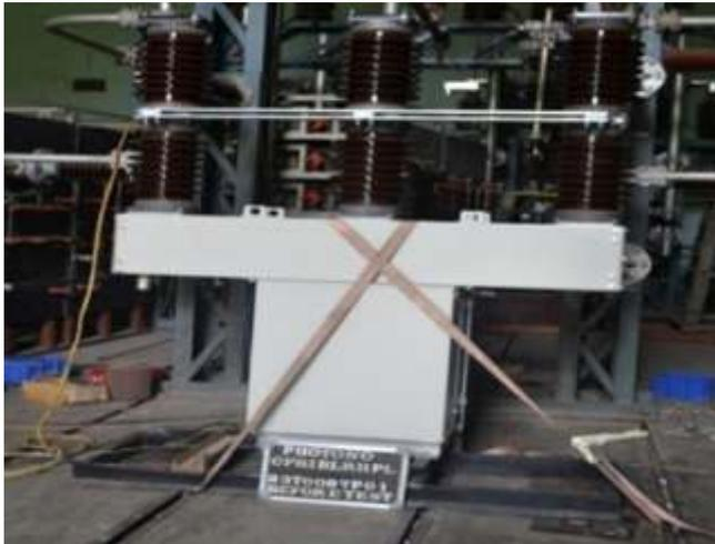
**Short Circuit test duties on 36kV, 31.5kA Three Phase Circuit Breaker by single phase method**
