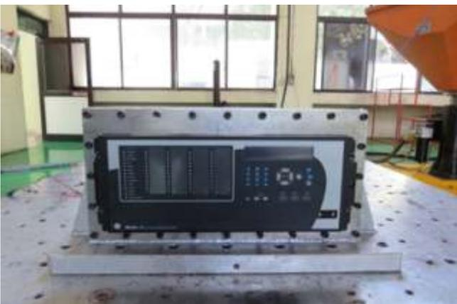
**Seismic test on Line Current Differential System**
