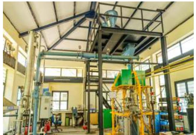
**Microwave Plasma Setup for Multi Fuel Gasification**
