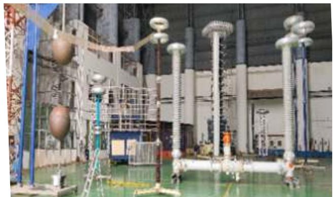
**Bias Test on 420kV GIS Isolator**
