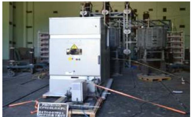
**Short Circuit making test on 36kV, 31.5kA Three Phase Earth Switch by alternative test method**
