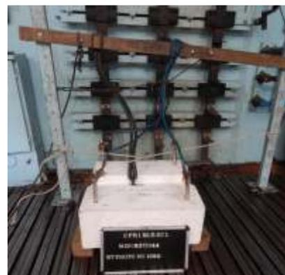
**Short-time withstand current and peak withstand current tests on RCC Earthing Block**
