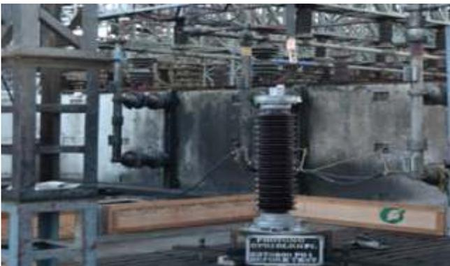
**Short Circuit test on 120kV Porcelain Surge Arrester for 50kA**
