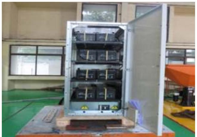
**Random Vibration test and Shock test on Battery Cabinet**
