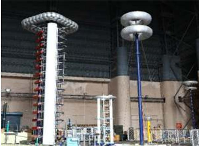
**Impulse Voltage Generator of 3MV, 150kj**
