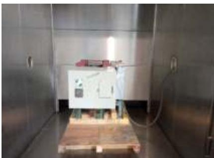
**Environmental Simulation test for Dry Heat and Damp Heat test on GIS Switchgear Control Cubicles**
