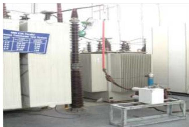
**Arrangement for Over Voltage Test on 200kVAR, 7.96kV, Internal HV Capacitor**
