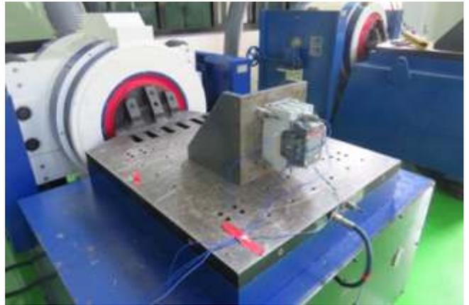
**Vibration and shock test on Contactors**
