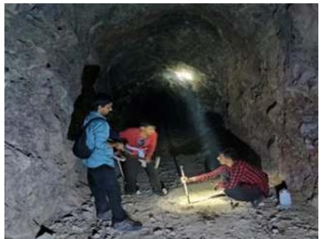
**Soil Resistivity Measurement as part of Design of Grounding System for 382MW Sunni Dam HEP**
