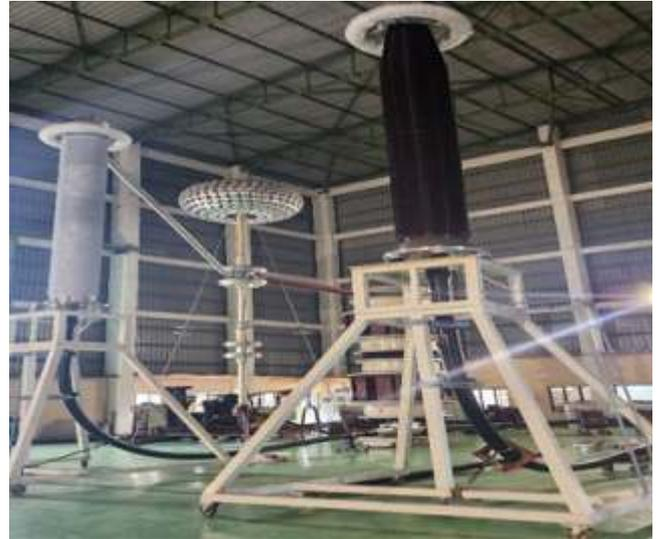
**Type test on 1X2500 Sq.mm, 400 kV XLPE Cable System**
