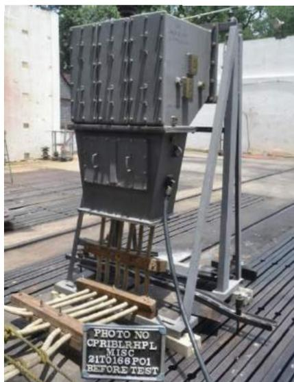
**Internal Arc test on 6.6/11kV PS Terminal Box**
