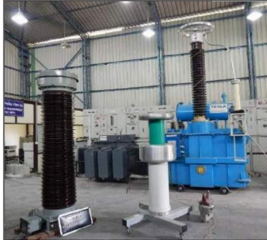
**Accuracy test on 220kV (ratio:  $220\text{kV}/\sqrt{3}:110/\sqrt{3}$ , 10VA, 0.2 class) Inductive Voltage Transformer**
