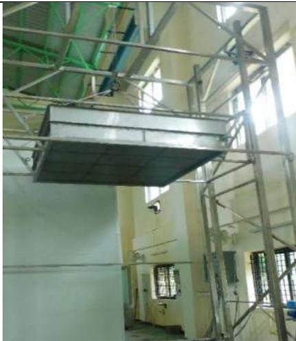
IP X1 and X2 test device
