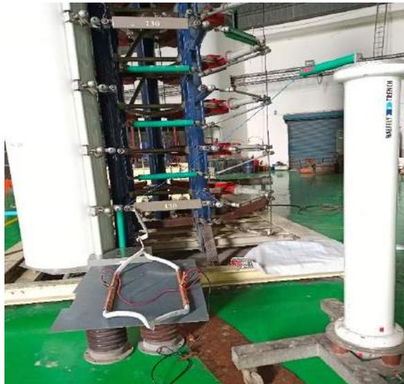
Impulse test on Inter turn Insulation of 11kV Motor Coil
