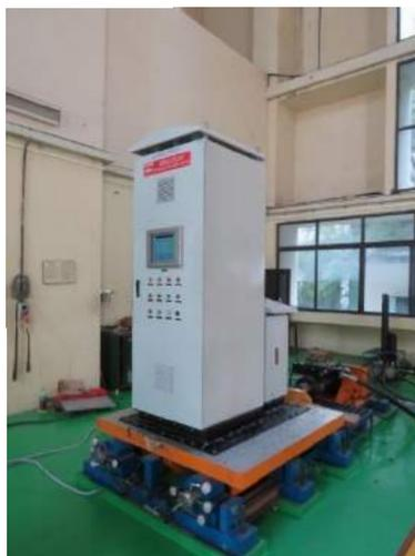
**Vibration testing of Local control panel and Remote Control Panel of Coal Feeder**
