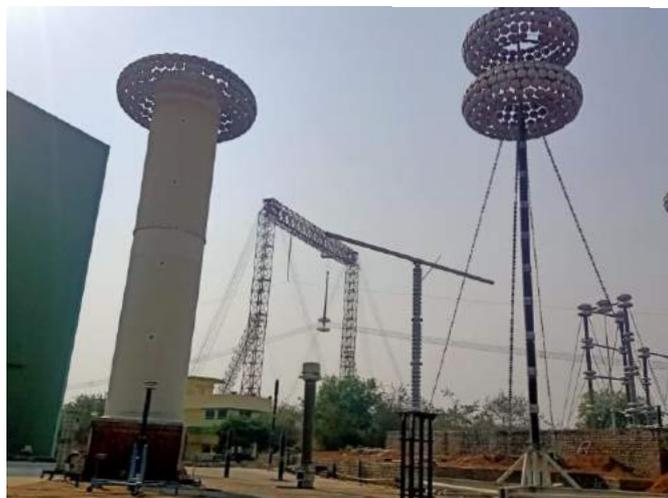
**Critical Impulse Flashover test on 525 kV, Porcelain Solid Core Post Insulator**
