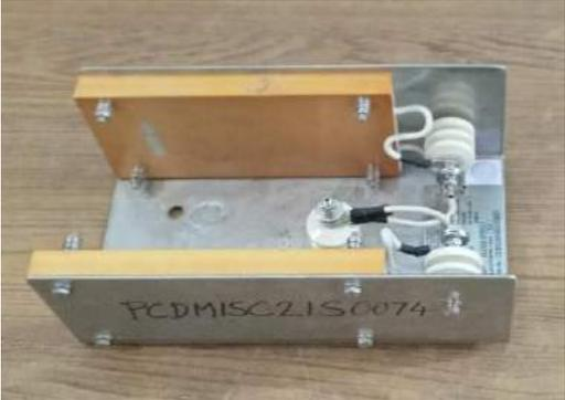
**A view of the discharge resistor**
