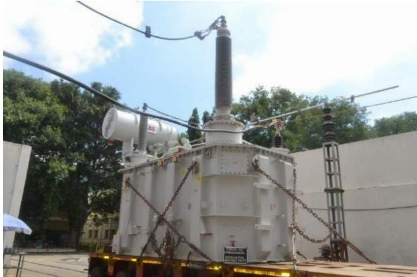
**Dynamic ability to withstand short circuit test on 53.33 MVA,  $220/\sqrt{3}/132/\sqrt{3}/33$  kV single-phase Transformer**
