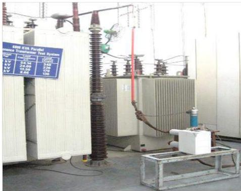
**Arrangement for Over Voltage Test on 110kvar, 3.608kV, Internal HV capacitor**
