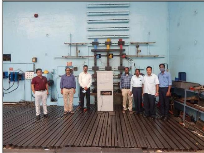
**Verification of short circuit withstand strength test at 31.5kA for 3s with 66.15 kA peak on main bus bars & 18.9 kA for 3s with 37.8 kA peak on neutral bus bar on 400V 1600A Ground mounted LV Metering KIOSK**
