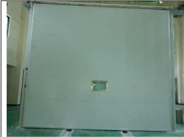
Dust chamber to accommodate DUT of size upto 4.5\*4\*4m (WDH)
