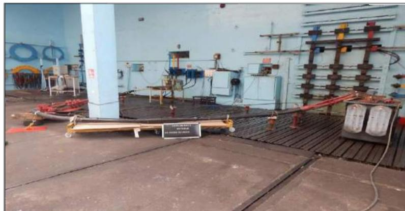
**Thermal short circuit test at 20kA rms for 1 second through screen & armour on 3 x 240 sq.mm Copper conductor, XLPE insulated PVC sheathed 18/30kV Cable with accessories (Heat Shrink Indoor Termination, Outdoor Termination and a straight through joint)**
