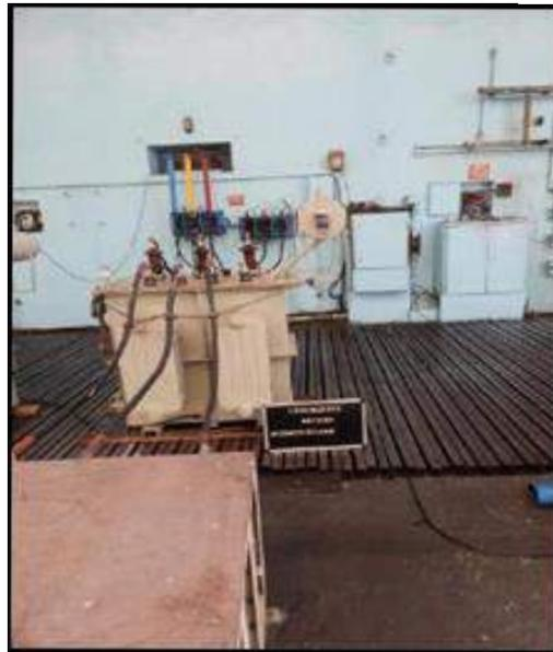
**Ability to withstand the dynamic effects of Short Circuit & Temperature Rise tests on 200kVA 11000/415V & 250kVA 11000/415V Three Phase Distribution Transformers**
