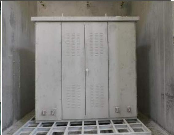
DUT in dust test chamber after IP 5X test
