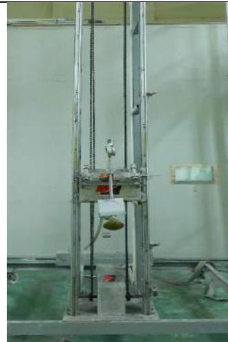
IP X3, X4, X5 and X6 test device with an auto movement of test nozzles
