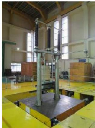
**Seismic qualification test on 132 kV, 2000A Disconnecter**
