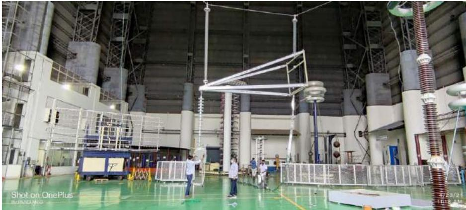
**Lightning Impulse voltage withstand Test, Dry & wet Switching Impulse Voltage withstand Test, Dry & Wet and Power Frequency Voltage withstand Tests on 132kV /23L VMCC FRP Composite Cross Arm**
