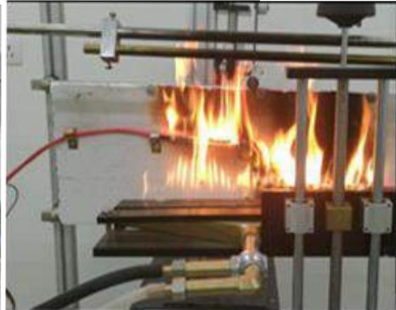
**Resistance to Fire with mechanical shock**
