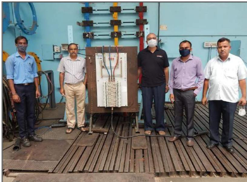
**Verification of short circuit withstand strength at 17kA for 0.25 s with 34 kA peak on main bus bars, at 10.2kA for 0.25 s with 20.4 kA peak on neutral and earth bus bars on 415V 160A 12 Way LV Distribution Board**
